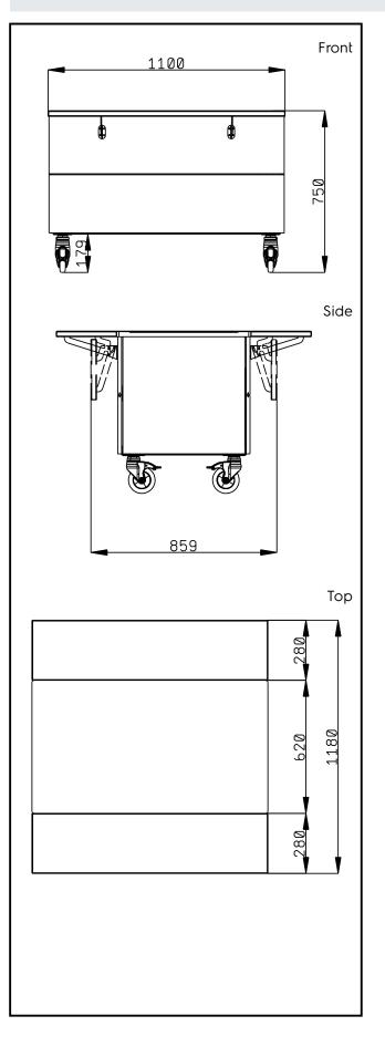
Flexy Compact Ambient Unit on cupboard (3 GN) with wheels and two stainless steel tray sliders, H=750mm The company reserves the right to make modifications to the products without prior notice. All information correct at time of printing.
